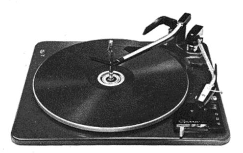
The low mass tubular pickup arm designed specially for use with high compliance cartridges is a special feature of this unit. This technique enables the actual performance of the cartridge to be obtained unimpaired by the mass or resonance of the arm and the pickup tracking characteristics reduce record wear to a minimum.
