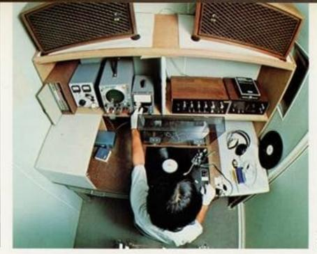
Testing and aligning a turntable inside a shielded room
