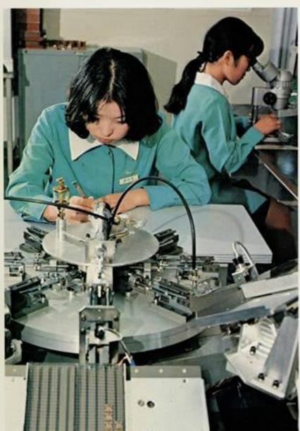
Sansui-developed automatic head core inserting machine
